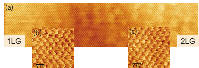
FIG. 7. (Color online) (a) High spatial resolution lateral force map recorded on a sample region with a transition between 1LG and 2LG films. (Image size: 25 \times 5.7 \text{ nm}^2 .) (b) Magnification of data on the 1LG region in (a). (c) Magnification of data on the 2LG region in (a).
